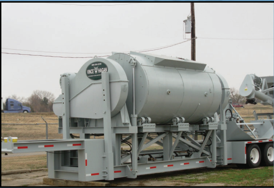
Portable RCC Horizontal Mixer in Travel Position
