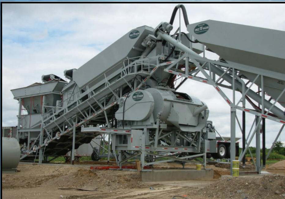
Portable RCC Horizontal Mixer with HT Plant and HCA
